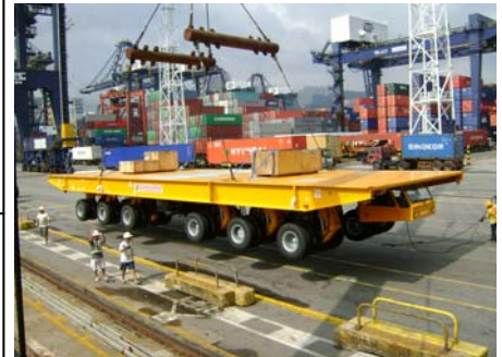
Loading operations of the transporter onto a feeder barge.
